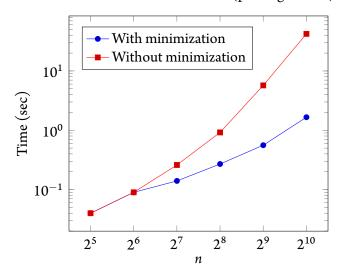
**Figure 6.6:** Minimizing goals is essential to achieve good asymptotic performance when tactics generate many unification variables. The time represents only computation time, not the time for reification.
